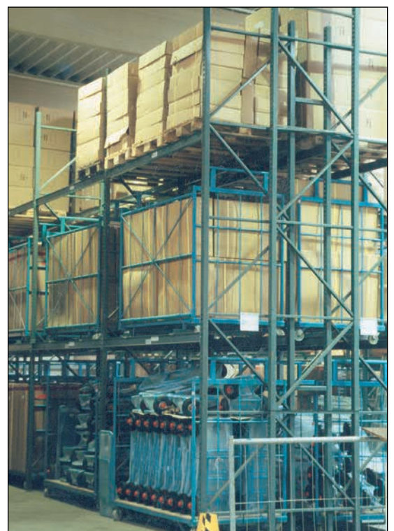
Stored in special racking 750-800 mm deep support bars
