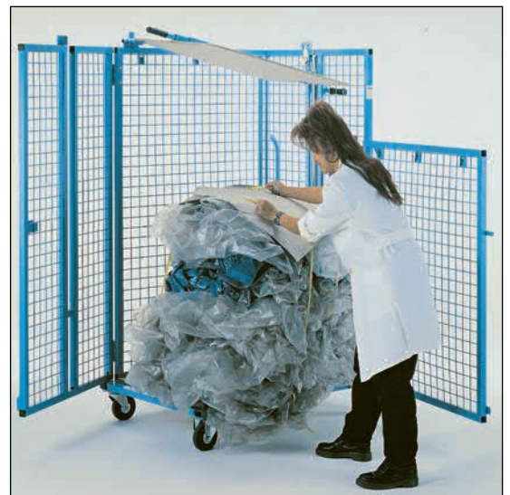
Banding after compressing.
